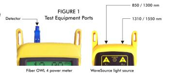
NOTE: the diagrams in this guide show singlemode. To use these instructions for multimode, simply use a multimode cable in place of the singlemode and make sure to use the multimode port on the light source.
