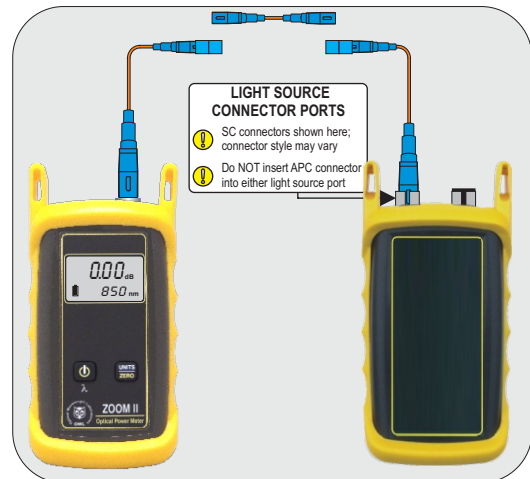
Insertion Loss Test
