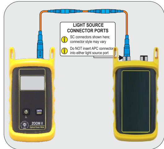
3-jumper Reference Method Setup
