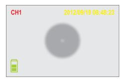
Using the focus adjustment wheel on the probe, focus the image on the LCD display.
