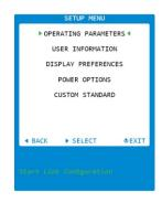
SETUP MENU > OPERATING PARAMETERS -- set length units and index of refraction
