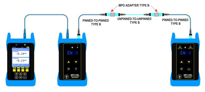
NOTE: for automatic channel switching to function properly, the bluetooth connection between the switch and the meter must be set up.
