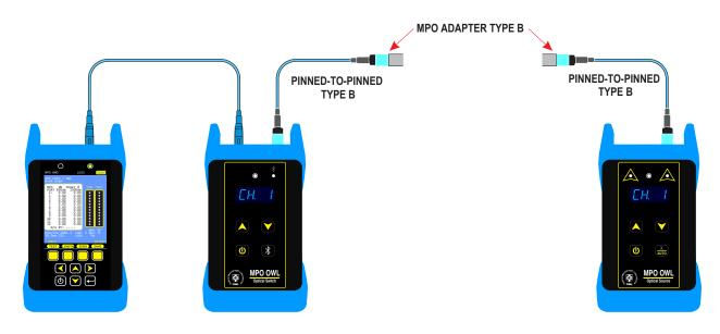
3) Insert the next cable under test, then press TEST.
