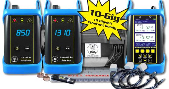
Power Meter: Fiber OWL 7 (p/n: F7) Light Source: Dual OWL Pro 850 (p/n: DP8X) Laser OWL Pro 1310 (p/n: LP3X) Patch cables, adapters, and other related accessories not included.
