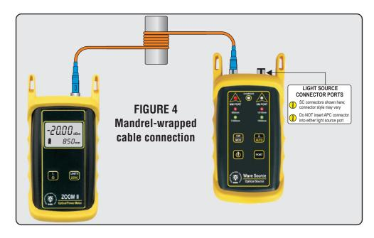
Compare the reading on the ZOOM 2 to Table 1 for acceptable power levels. The mandrel-wrapped patch cable should be replaced if it is below the acceptable power level.
