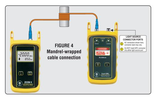
Compare the reading on the ZOOM 2 to Table 1 for acceptable power levels. The mandrel-wrapped patch cable should be replaced if it is below the acceptable power level. Once proper operation has been verified, remove the mandrel-wrapped cable from the power meter and light source, then continue to the next step.
