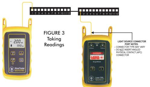
**STEP 19** Press  $\lambda$ /AUTO several times until the WaveTester is set to 1310nm.
