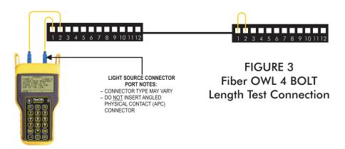
**STEP 23** Review the end-to-end fiber length. In the example screenshot at right, the end-toend fiber length could be within the range of 1000 to 1006 meters.
