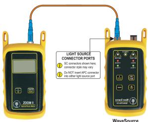
WaveSource connected to 850nm port
