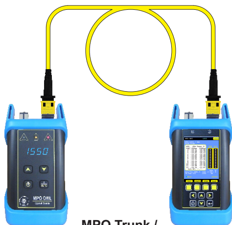
MPO Trunk / Patch Cable Testing
